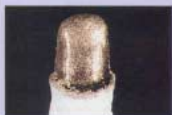
Figure 5—Finished coping coping. Note the warm gold color and diffuse reflective surface.
